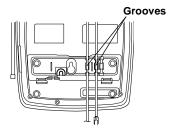
6. Align the bracket's keyhole slots with the mounting screws and slide the base downward to secure it.
